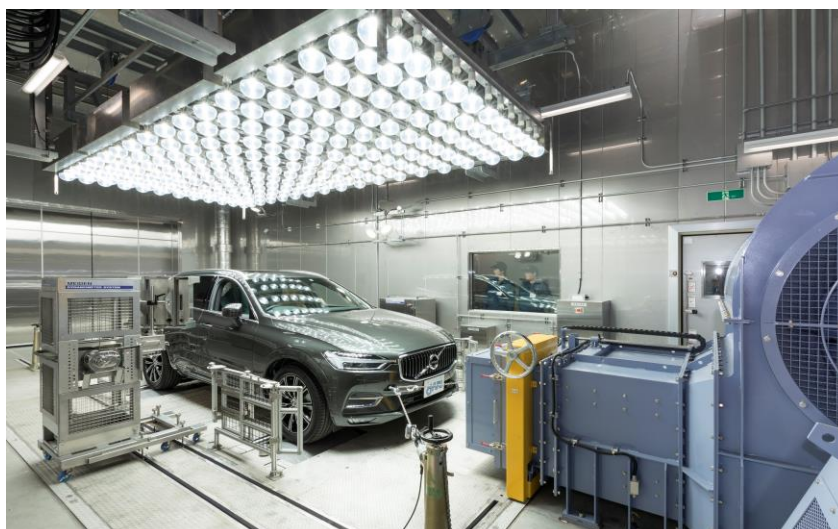
Fig. 5 Appearance of the environmental chasis dynamometer.
