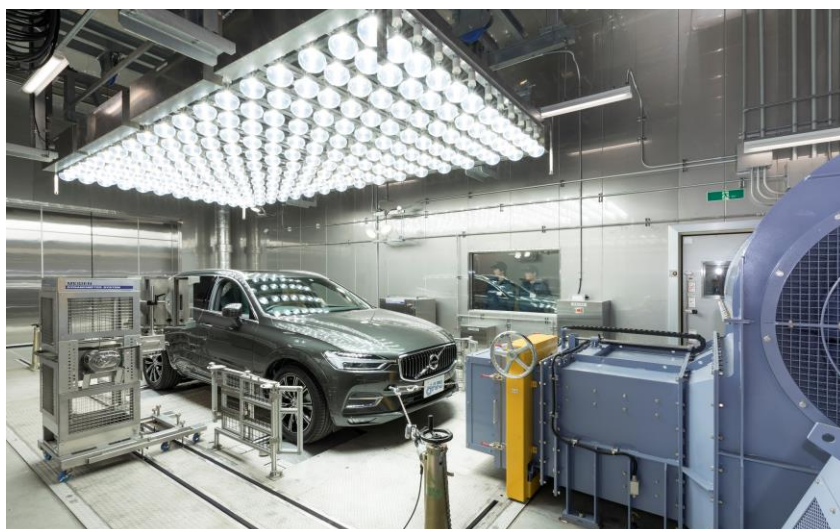
Fig. 5 Appearance of the environmental chasis dynamometer.
